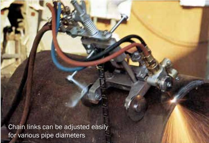
Chain links can be adjusted easily for various pipe diameters
