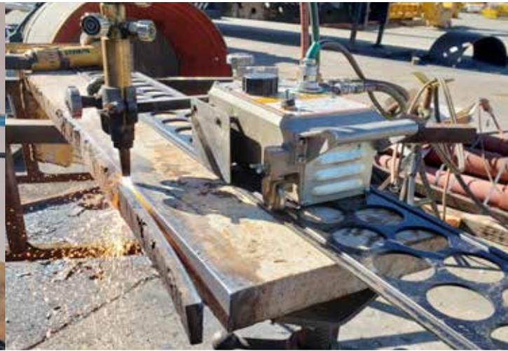
The IK-12 Beetle is an affordable, portable, oxy-fuel cutting machine. It is known around the world as one of the best portable cutting machines in the industry.
